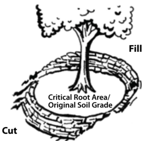
**Figure 10.** Retaining walls can keep original soil grade within the critical root area and allow deep cuts and/or fills to achieve the grade changes needed for construction.
