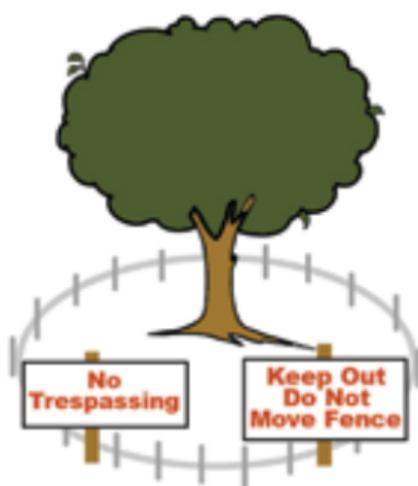
**Figure 6a.** Placing a protective fence around the critical root area assures tree survival.
