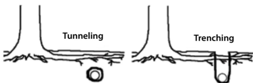
**Figure 9.** Utility lines may be placed near trees without root injury by tunneling underground. An alternative is trenching with a pneumatic air excavator or careful hand digging.
