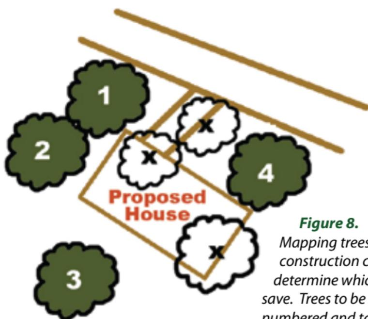
**Figure 8.** Mapping trees before construction can help determine which trees to save. Trees to be saved are numbered and tagged. Trees to be removed are marked with an x.
